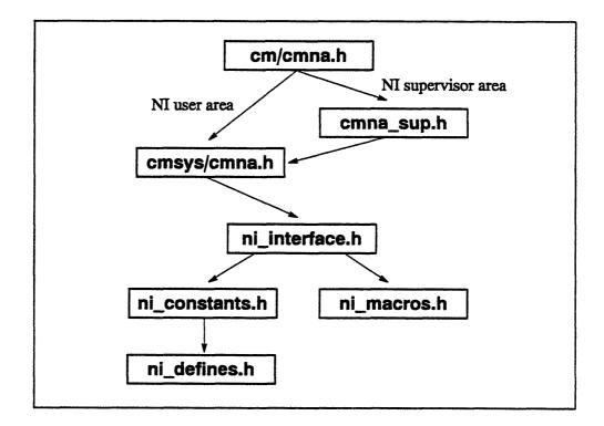
Figure 9. Relationship between CMNA and NI header files.
