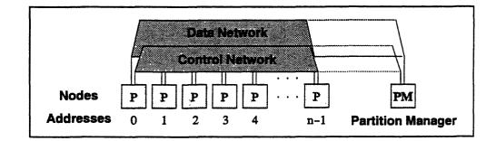
Figure 6. Addressing of nodes in a partition.
